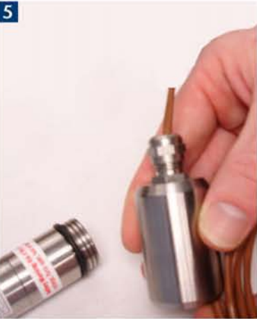
Figure 4 – Pull the thermocouple out of the thermo cover.
