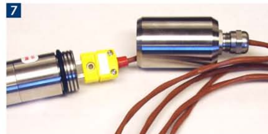
Figure 6 – The new thermocouple inserts into the body of the data
