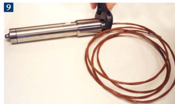
Figure 8 – Tightening the cable gland nut.
