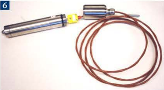
Figure 5 – Slide the new thermocouple sheath-first.
