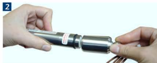
Figure 1 – Removing thermo cover from TCTemp1000 data logger body. Note the right hand is holding the cable gland, and the thermo cover is being removed from the TCTemp1000 data logger
