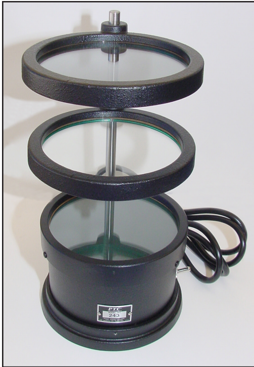
Model 243 6" Polariscope Tint Plate is located between the analyzer ring and polarizer
